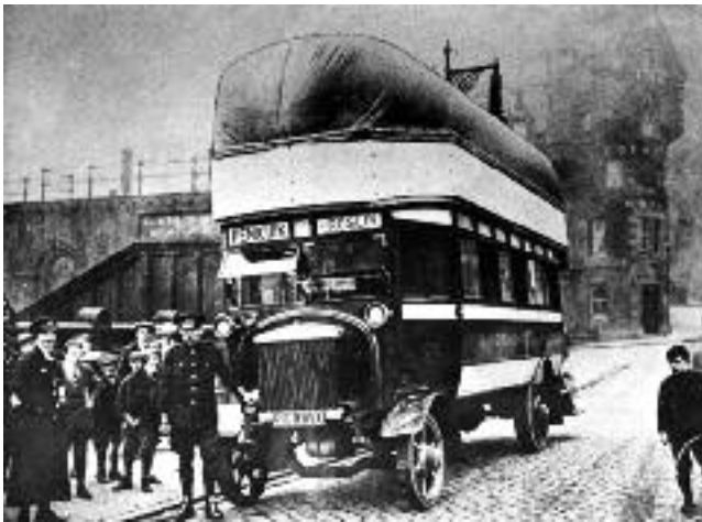
Shortage of petrol led to some public buses being adapted to run on coal gas. Bags were attached to the roof, and they gradually shrank as the fuel was used up. As someone remarked at the end of the war: 'it seemed a good idea at the time.'
